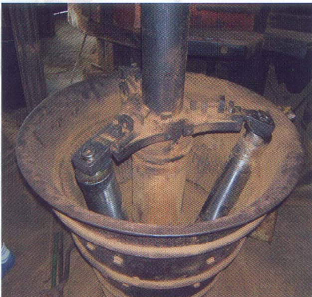
Above: one of the old snuff mortars at Samuel Gawiths Kendal Brown House. Below: the water-driven mill of Wilsons and Co (Sharrow) in Sheffield.
