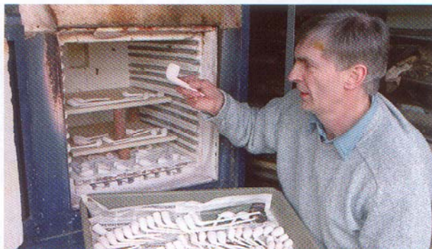
Clay pipes are fired in a kiln to harden them.
